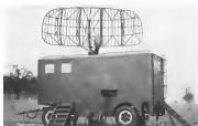
MOBILE RADAR target acquisition radar is key portion of equipment of division level, covers the three missile batteries of the division. Laboratory comes from early writing order set in the unit, a three piece along to proper missile battery.
